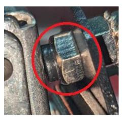
The hole to be drilled should have a diameter of 15mm to create a recess for the 11mm nut. This recess is essential to ensure that the nut only tightens against the Light Bracket.
