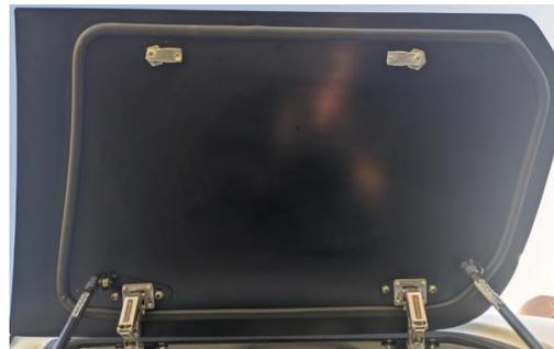
Once the door has been marked and primed, the weather seal can be attached to the door following outside of the marked lines so the seal will line up on the frame (if the seal does not correctly align, moisture and dust will find its way into the back of the vehicle).
